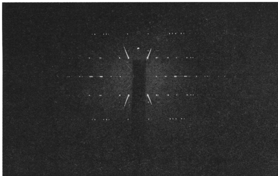
Plate 1. Oscillation photograph of the X-ray diffraction pattern exhibited by crystals of compound 18.
